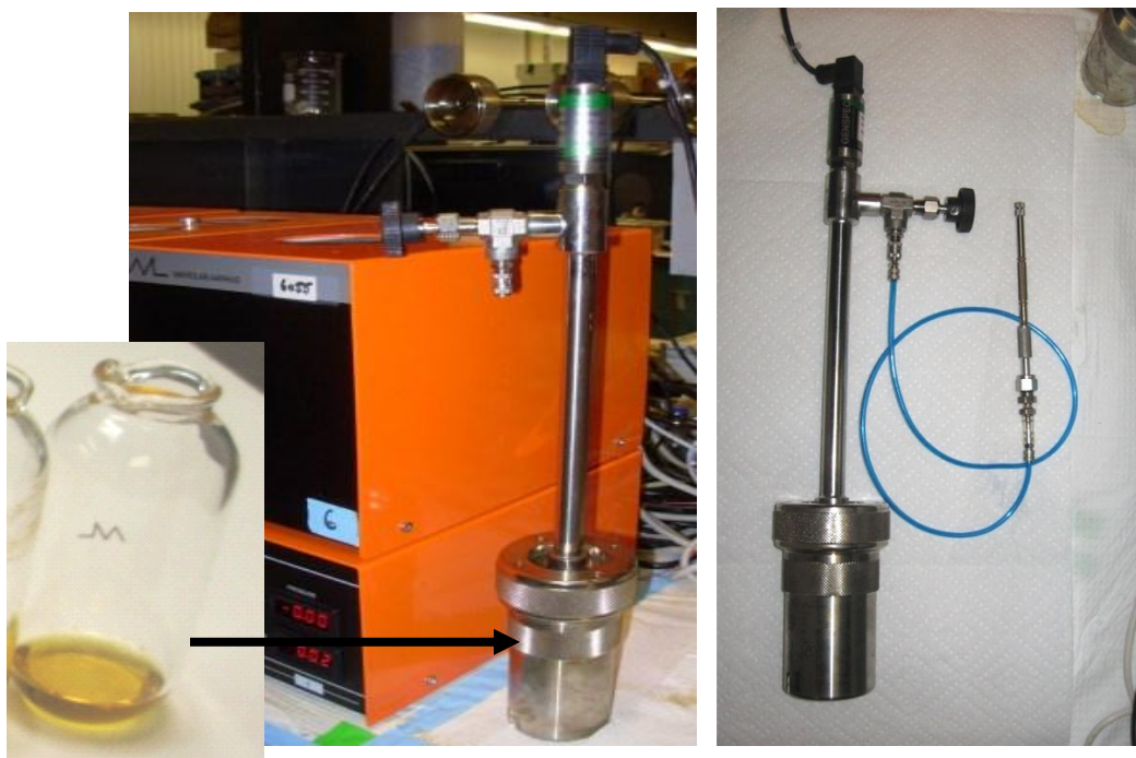
Figure 11. Oxipres™ oxygen bomb instrumentation. Left: Heating block, sample vial, and pressurized sample cell. Right: Connection of sample cell to Tenax trap for collecting vented volatiles upon release of pressure on cell.
