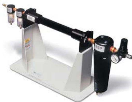
Figure 3. Filtered Air Supply. From left to right: two coalescing filters (DX and BX grade to remove water/oil and particles), membrane dryer to remove moisture, a final carbon-vapor filter to absorb any remaining oil vapors, and gas regulator for pressure
