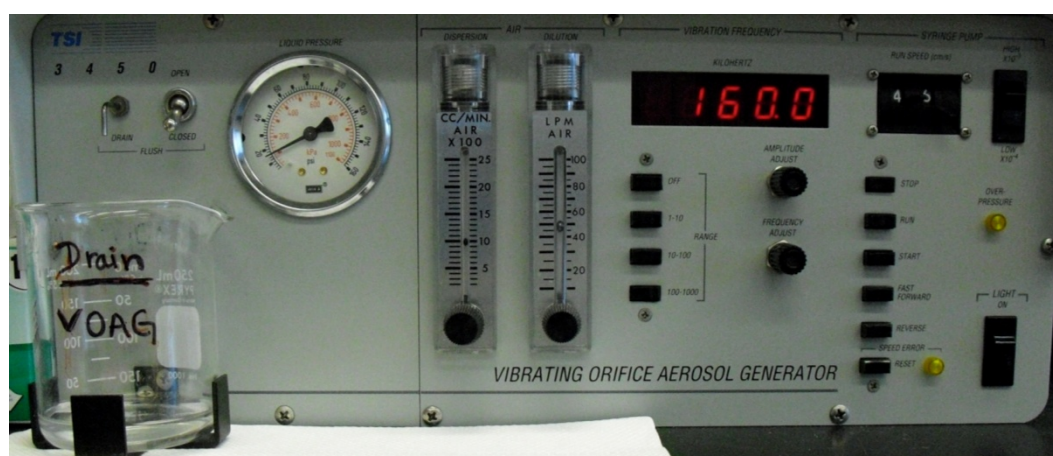
Figure 2. VOAG's Front Panel Controls and Indicators. (Power button on the back)
