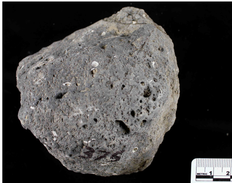
Figure 3.3: Examples of (a) fine grained basalt (core number 350) and (b) vesicular basalt (core number 375) from Olduvai Gorge, Tanzania.
