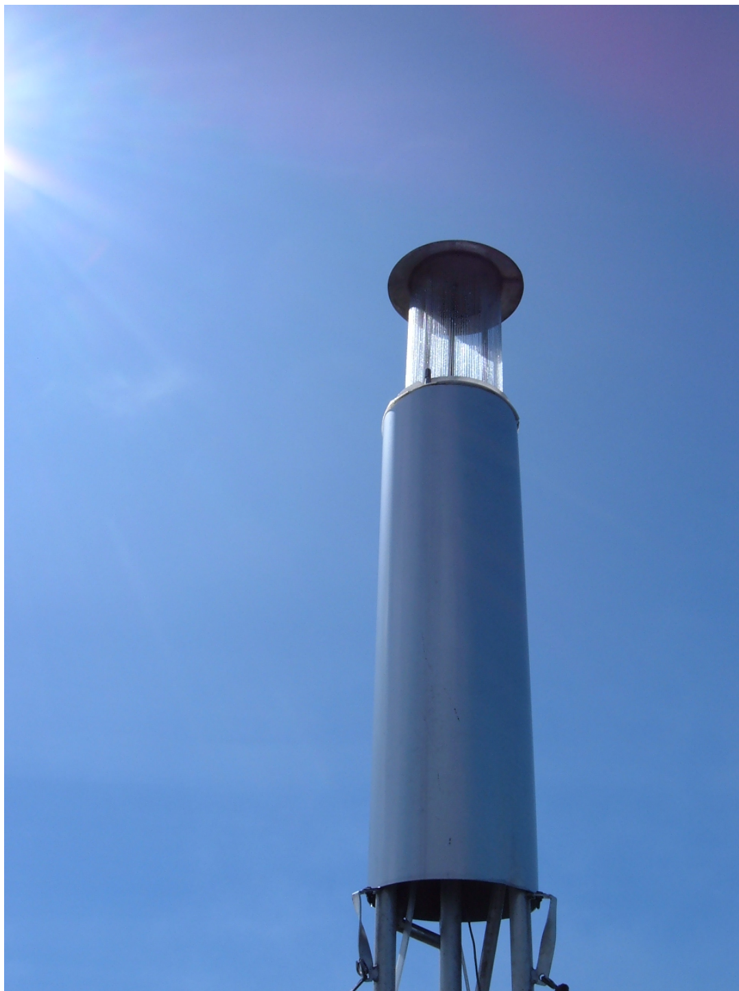
Figure 3.3. The cloud water collector in collection mode. Photo taken August 24, 2010 by the author.
