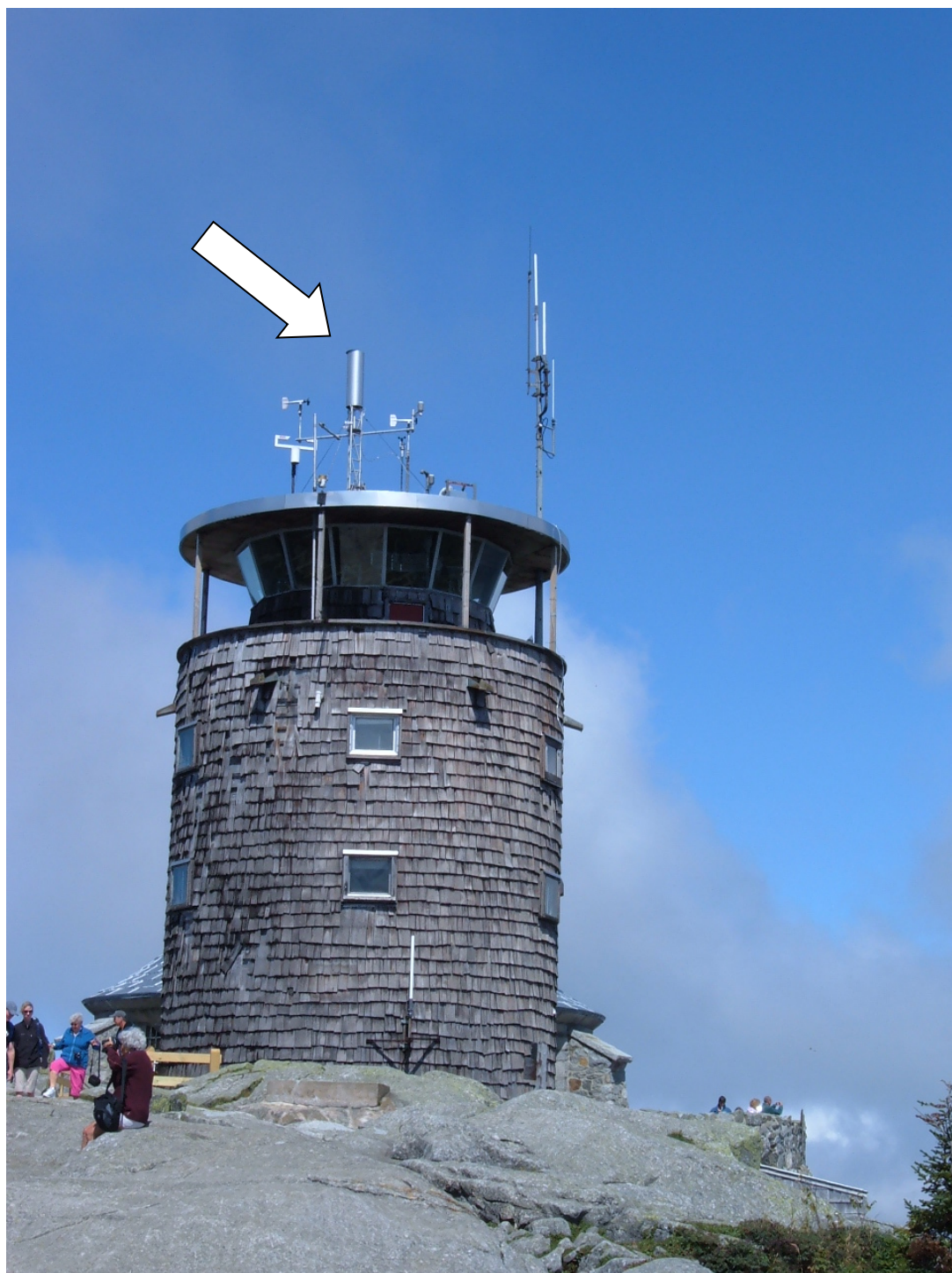
Figure 3.2. Cloud water collection station, Whiteface Mountain. The cloud water collector is indicated by the arrow. Photo taken August 24, 2010 by the author.
