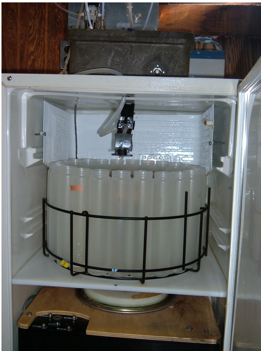
Figure 3.4. Cloud water collection bottles inside a refrigerator. The tubing at the top is directly connected to the cloud water sampler. Photo taken August 24, 2010 by the author.
