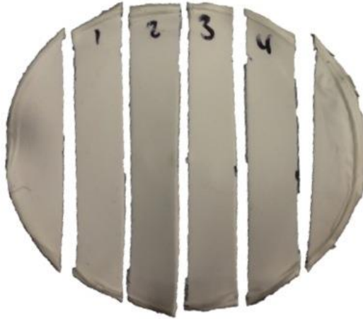
Figure 3-8: Preparation of Electrospun scaffold for mechanical testing.
