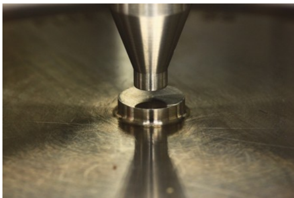
Figure 25 Parallel Plates for Size Comparison (4 mm Top, 8 mm Bottom)
