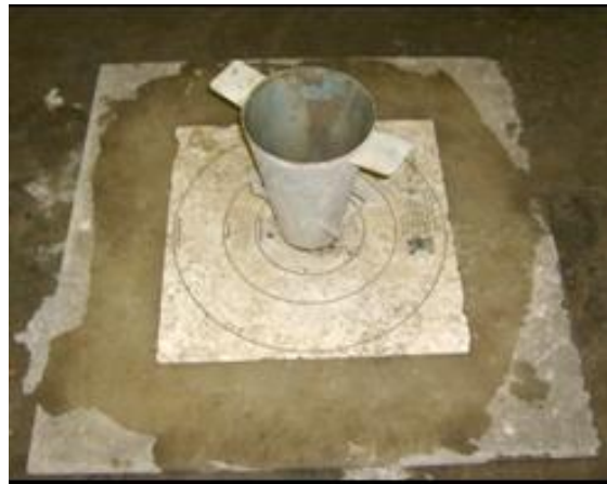
Figure 4.2: Slump flow test set up
