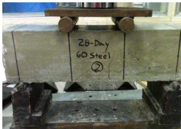
Figure 5.8: Failed beam of Steel60 after flexural testing
