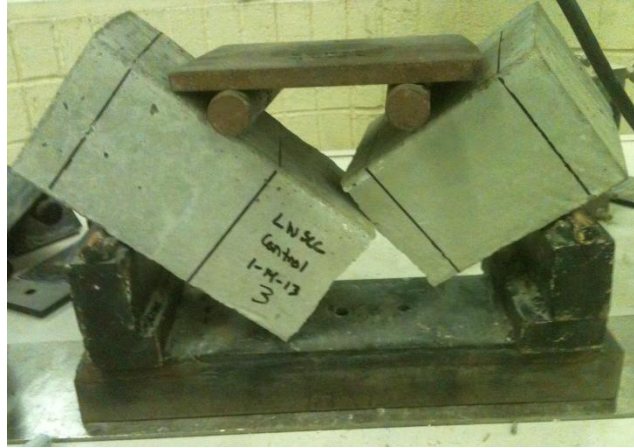
Figure 5.7: Failed beam of control after flexural testing
