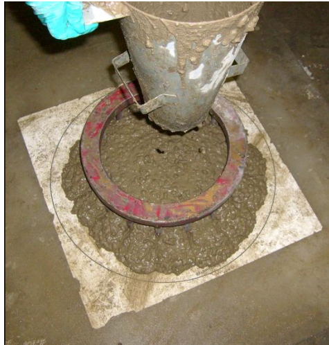
Figure 4.3: Passing ability test with J-Ring
