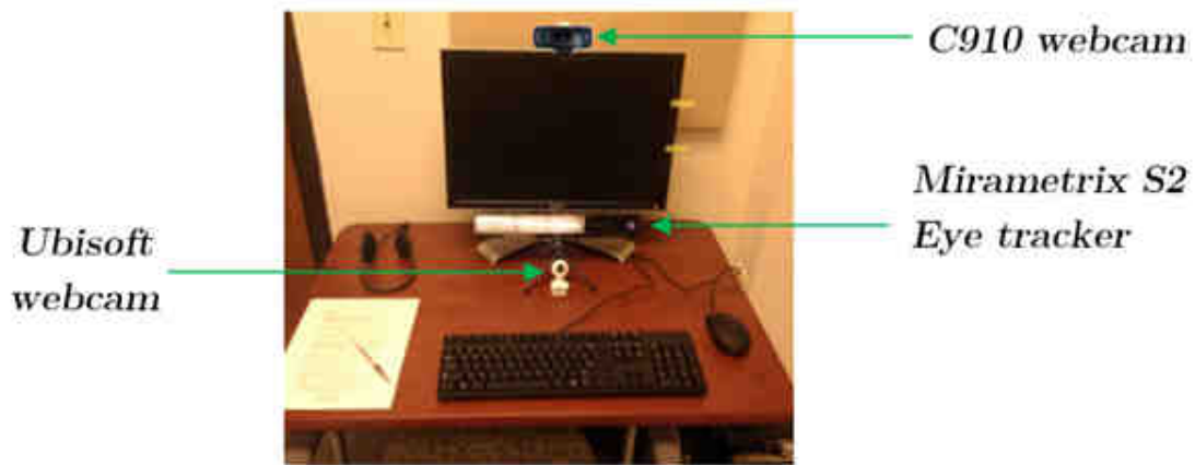
Figure 4.6. Eye tracker and webcams setup.
