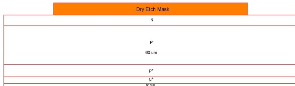
(b) Dry etch mask formation for Isolation
