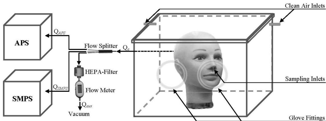
Figure. 3.1. Aerosol generation and analysis experimental setup for simulated application of the spray products (a) and constant output aerosolization (b).
