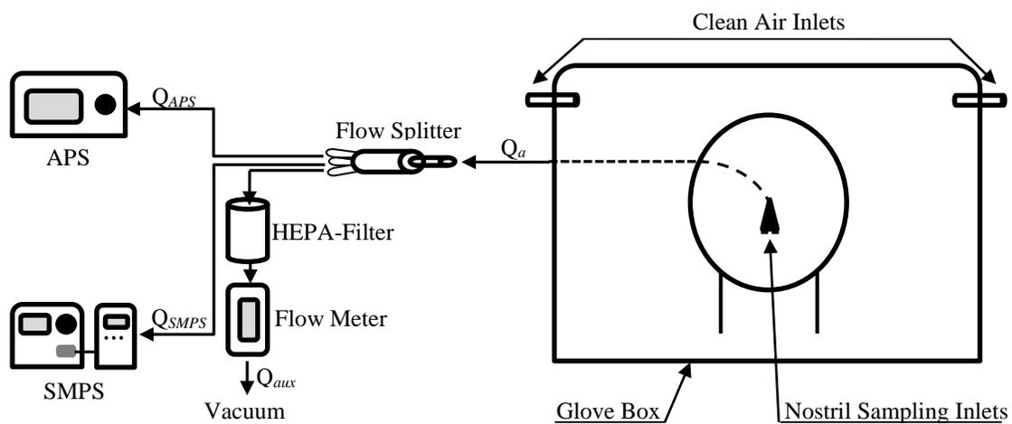
Figure. 4.1. Setup for exposure measurement of airborne particulate matter resulting from simulated cosmetic powder application.
