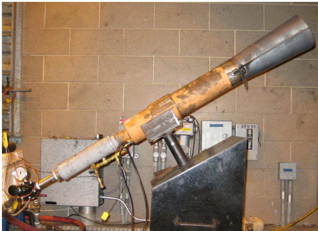
**Figure 2.17. Photograph of the FAA next generation fire test burner thermal acoustic insulation burnthrough apparatus.**
