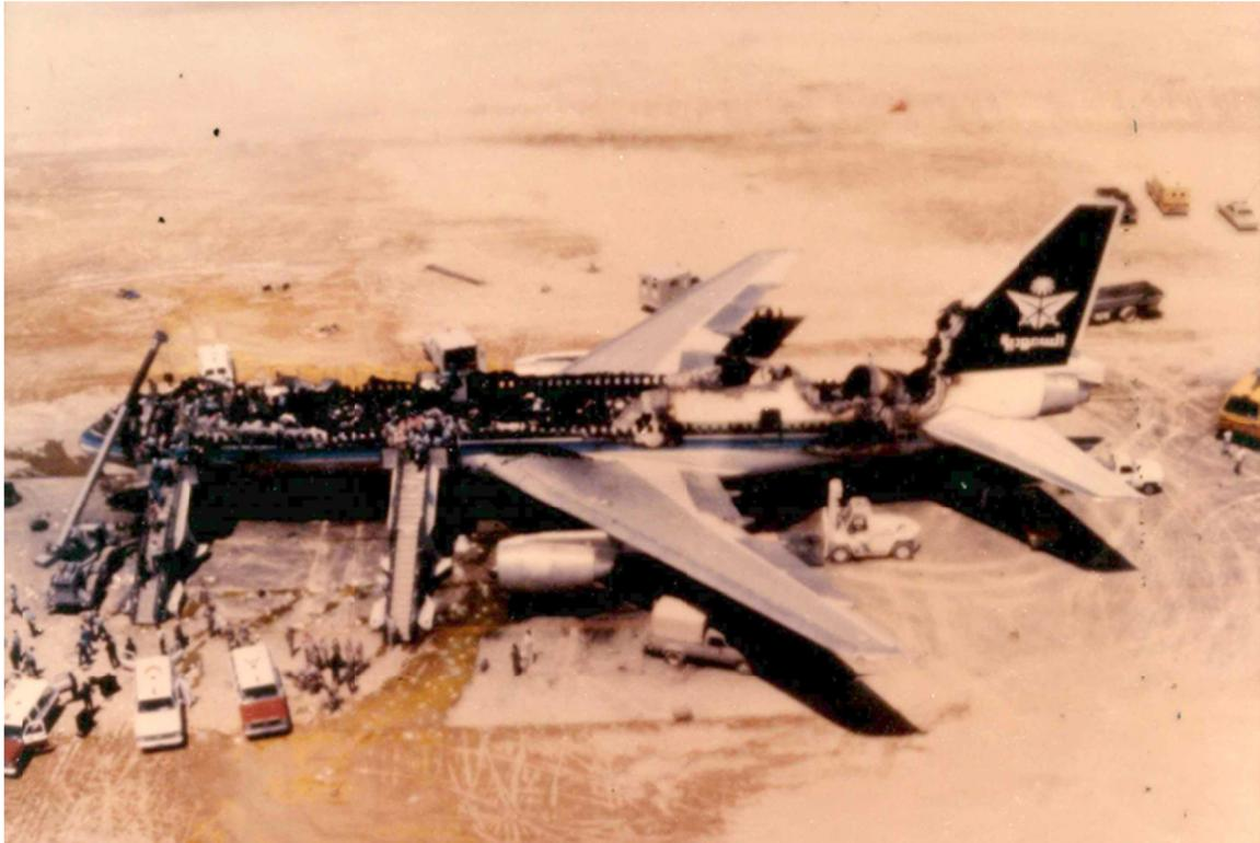
**Figure 1.4. Post-accident photograph of Saudi Arabian Airlines Flight 163 at Riyadh, Saudi Arabia, August 19, 1980. A fire originating in a class D cargo compartment breached the cargo lining materials, allowing oxygen to fuel the fire and flames to spread to the passenger cabin. The plane successfully landed but flashover occurred before evacuation was initiated. All 301 persons aboard perished.**
