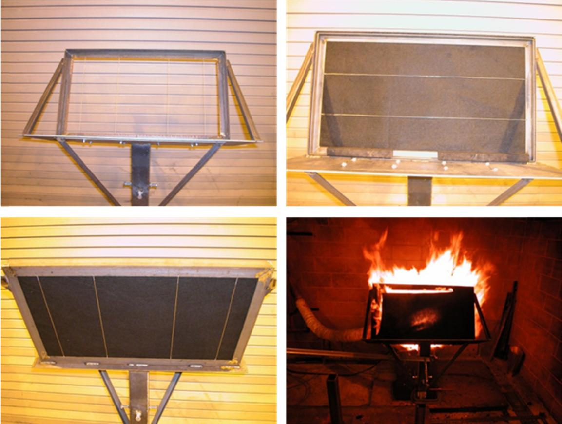
Figure 2.18. Photographs of the picture frame sample holder.
