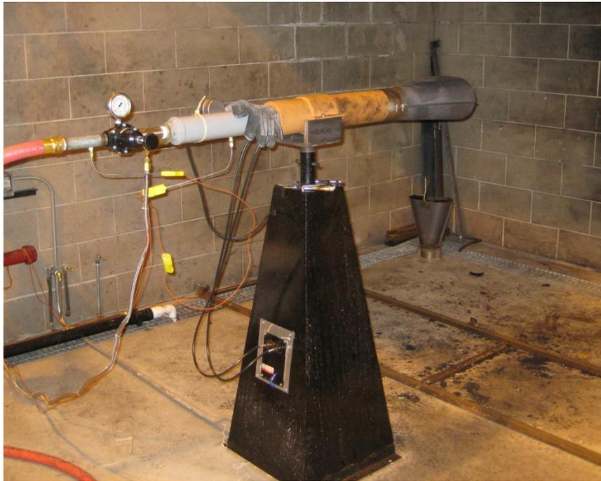
**Figure 2.15. Photograph of the FAA next generation fire test burner seat cushion flammability apparatus.**
