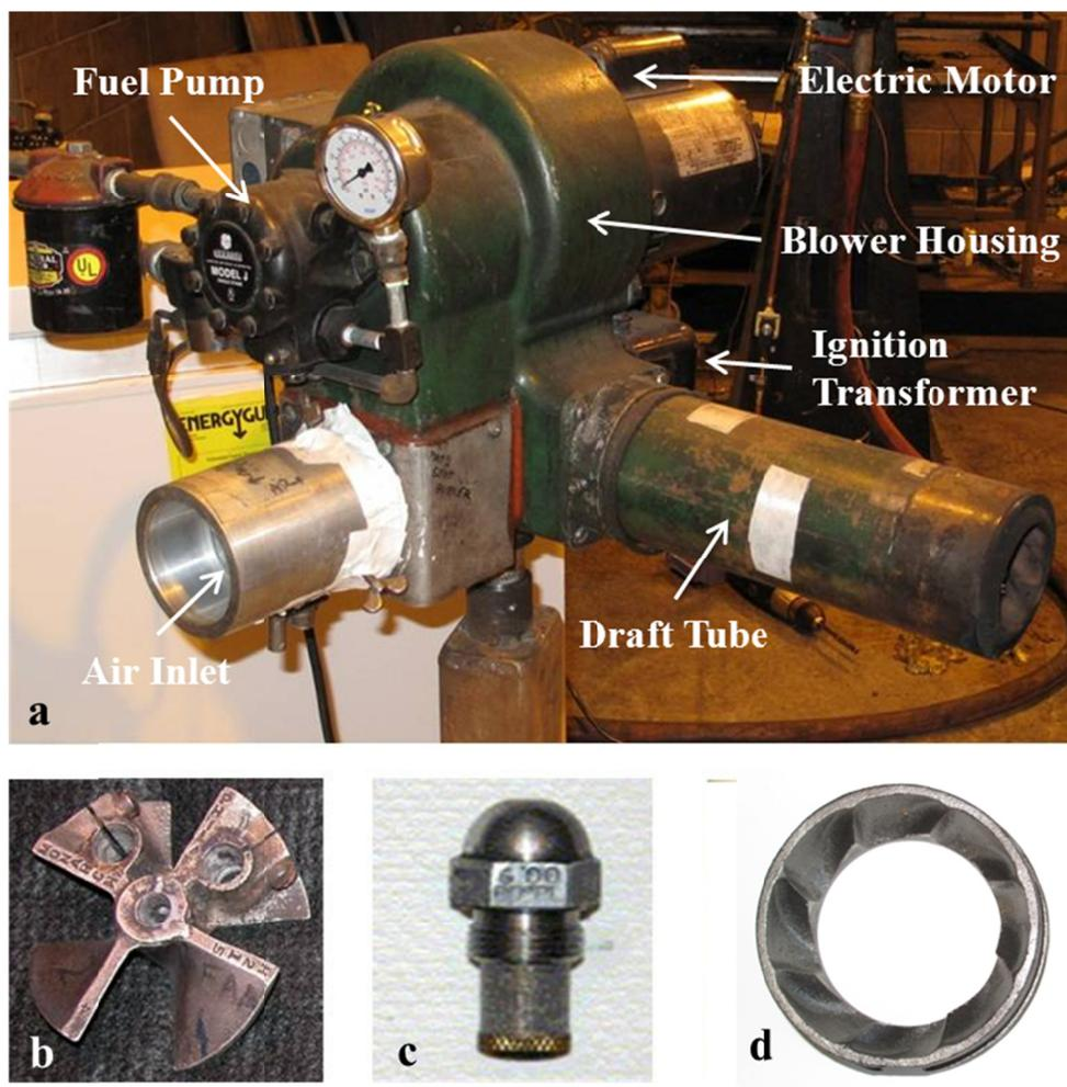
Figure 1.8. Park DPL3400 oil burner (a) and internal components stator (b), fuel nozzle (c), and turbulator (d).
