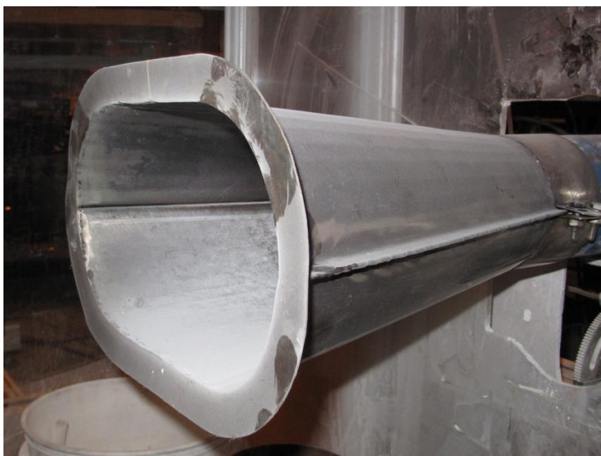
**Figure 4.27. Photograph of a reinforced burner cone.**
