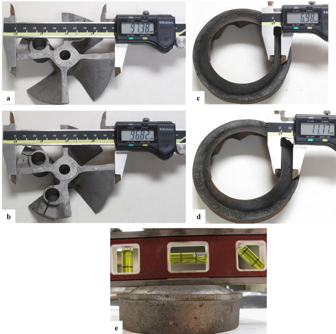
**Figure 1.14.** Photographs of the original stator (a,b) and turbulator (c-e). The stator is nominally 101.6 mm in diameter, but some castings are not to specification (a). The stator is also asymmetric about the center hole (a,b). The turbulator opening should be centrally located, but is cut off-axis, resulting in a skewed exit plane (c, d). The turbulator profile view in (e) shows the off-axis direction of the exit plane.
