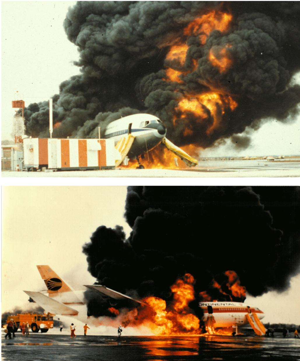
**Figure 1.2. Examples of post-crash fire accidents: ONA Flight 032 at JFK airport, New York, 1975 (top) and Continental Flight 603 at LAX, Los Angeles, 1978. The accidents are considered survivable in that the passengers are fully capable of exiting the aircraft, though the effects of the external fire on the cabin materials significantly reduce survivability time.**
