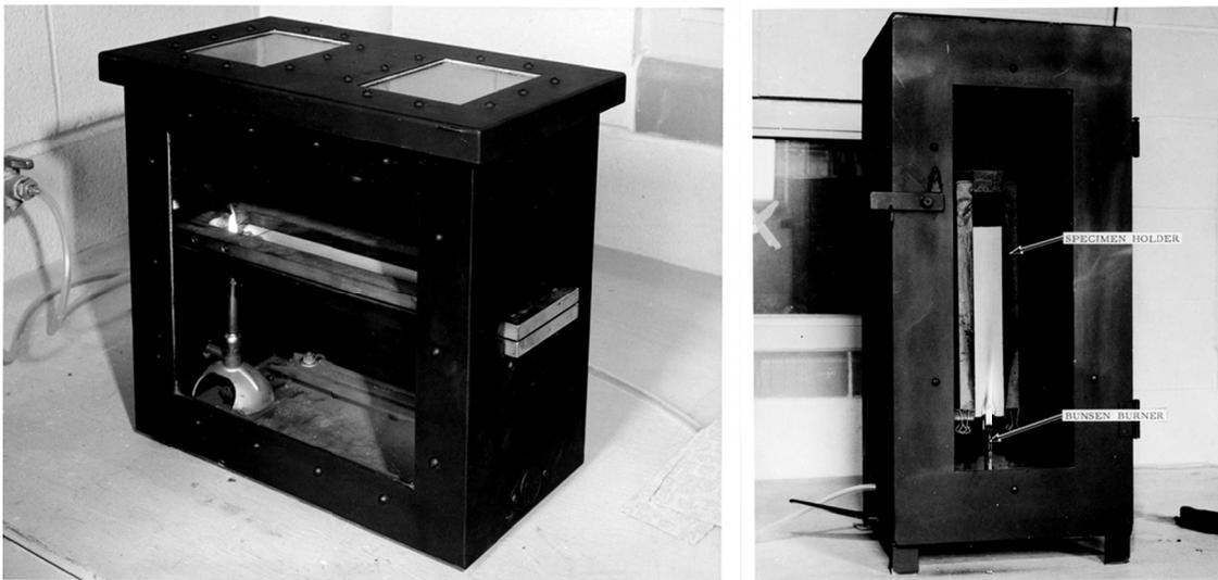
**Figure 1.1** Photograph of the original FAA fire test methods, the horizontal Bunsen burner (left) and the vertical Bunsen burner (right).
