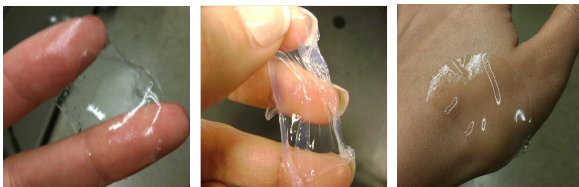
Figure 1.13. Formulation of salicylic acid-based polymers blended with PVP to create materials that exhibit hydrogel-like properties
