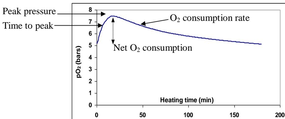
Figure 20. Typical Oxipres oxygen consumption generated when oils are heated to high temperatures (180 °C) under 5 bars oxygen pressure. Slopes and oxygen consumption decrease at lower temperatures and oxygen pressures.
