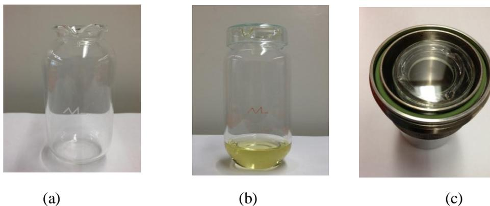
Figure 17. (a) An Oxipres™ sample flask; (b) oil deposited in the flask; (c) flask placed in pressure vessel. Glass lid is place on top of flask during heating to prevent contamination to oils.
