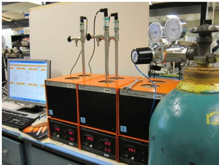
Figure 16. Oxipres oxygen bomb system with three samples running in individual positions of the control units. A gas supply and computer connect to each oxygen bomb cell.
