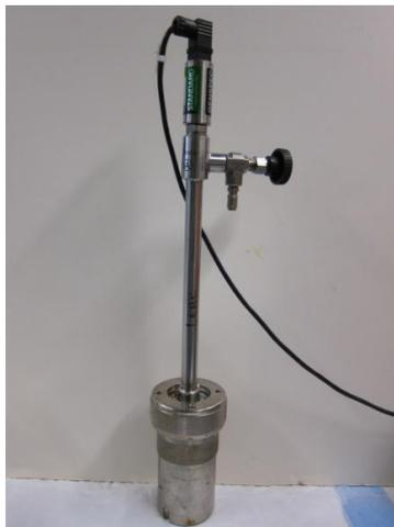
Figure 18. An Oxipres™ pressure vessel with pressure transducer (on the top) and signal transmitting lines.
