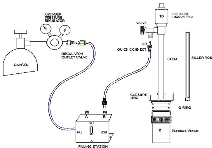
Figure 19. Scheme for pressurizing Oxipres™ pressure vessels.
