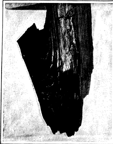
Same Branch split in half—Showing How Decay Undermined the Top
