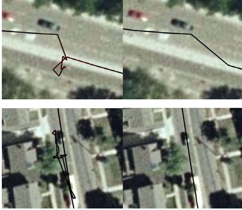
Figure 2.7: Trace before (the left two pictures) and after (the right two pictures) path smoothing pre-processing.
