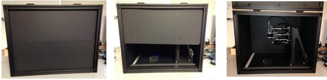
Figure 10: Light-tight casing around the prototype MI system
