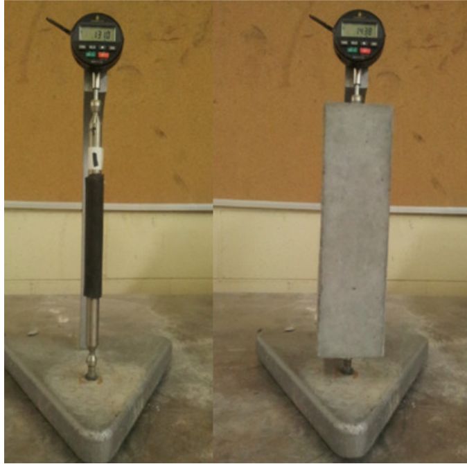
Figure 3.11 Length Comparator with Reference Bar and Prism
