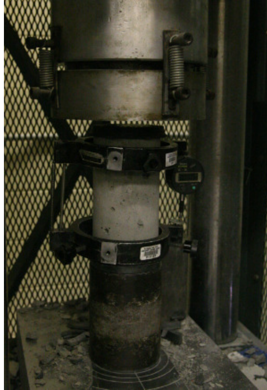
Figure 3.10 Compressometer Attached to Cylinder
