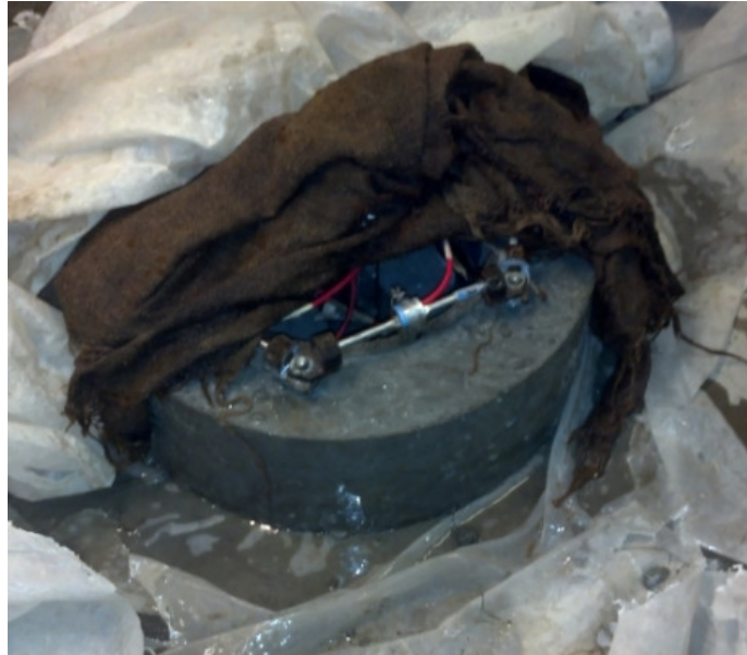
Figure 3.6 Wet Burlap Curing for AASHTO Ring
