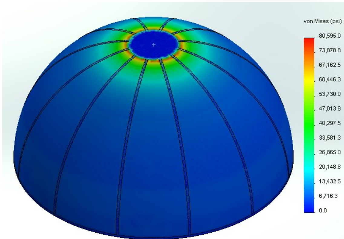
Figure 48: von Mises Stress Results for Static Tensile FEM of Thrust Structure and Reaction Chamber
