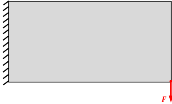
Figure 2.1. A Typical Selection of Design Domain in Topology Optimization
