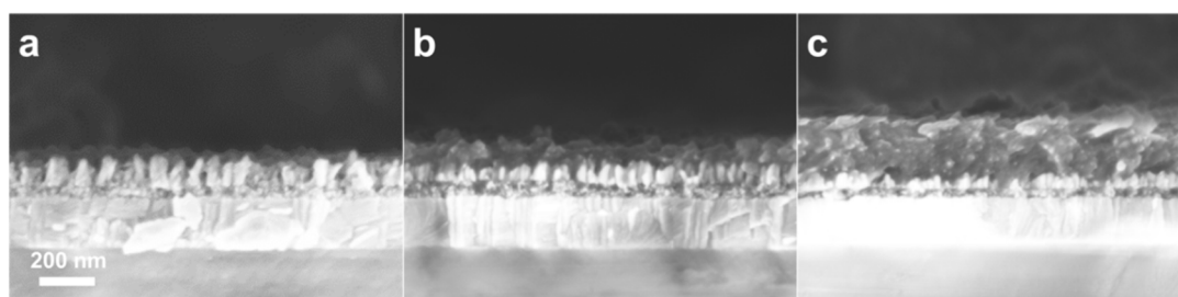
Fig. 4-3-6. Cross-sectional SEM images of e-PT on ZnO nanorods at an electrochemical charge of (a) 8 mC, (b) 25 mC and (c) 75 mC. The solvent used in electropolymerization is acetonitrile (ACN)
