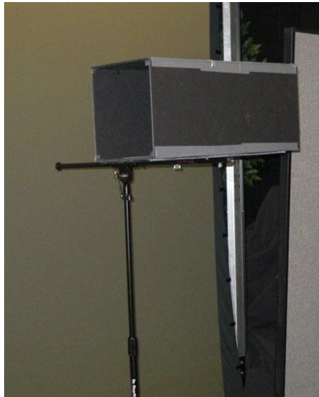
Figure 33. The tunnel used in the dart throwing condition, blocking vision of the throwing arm. The tunnel is 15 inches long and is large enough for participants to place their face in the opening. The tunnel was attached to a microphone stand to adjust for participants of various heights.
