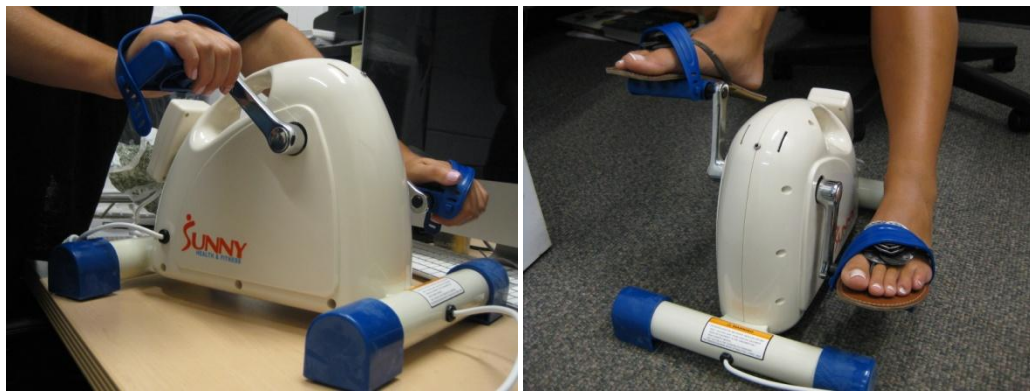
Figure 23. Photographs of the mini bike used for the motor manipulations in Experiment 3. Participants either actively or passively performed hand pedaling or active feet pedaling during the observation phase.
