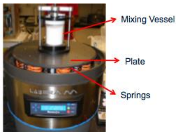
Figure 3-1. Laboratory scale resonant acoustic mixer (LabRAM) with 236-mL mixing vessel used in all experimental studies.
