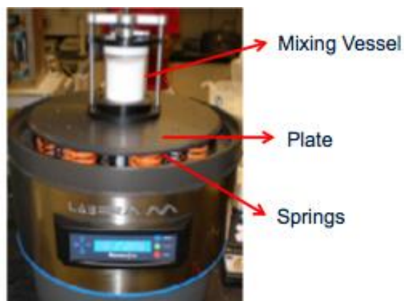
Figure 4-1. LabRAM with 236-mL mixing vessel.
