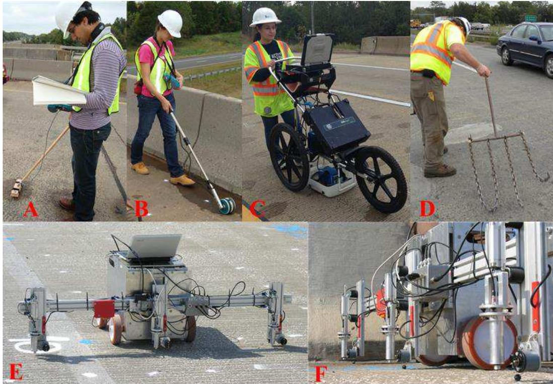
Figure 11: Non-destructive testing of a bridge deck, A) electrical resistivity, B) half-cell potential, C) ground penetrating radar, D) chain drag, E & F) impact echo
