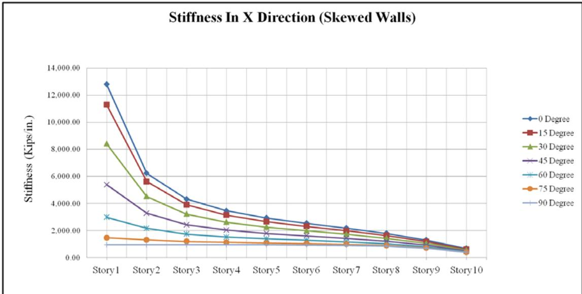
Figure 5.9: Stiffness comparison in X direction - skewed walls
