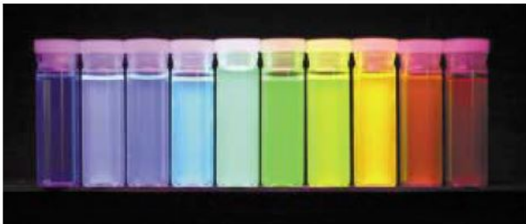
Figure 1.19: Ten distinguishable emission colors of ZnS-capped CdSe QDs excited with a near-UV lamp. From left to right (blue to red), the emission maxima are located at 443, 473, 481, 500, 518, 543, 565, 587, 620, and 655 nm. Reprinted from Ref. [82]. Copyright 2002 Elsevier, Inc.
