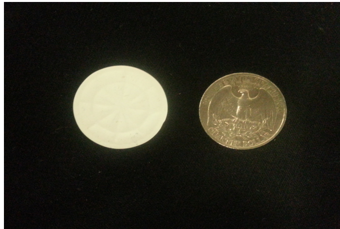
Figure 3.4: Supor®filter: Diameter - 25 mm, Pore Size - 0.2\mu\text{m} ., Thickness - 145\mu\text{m} .
