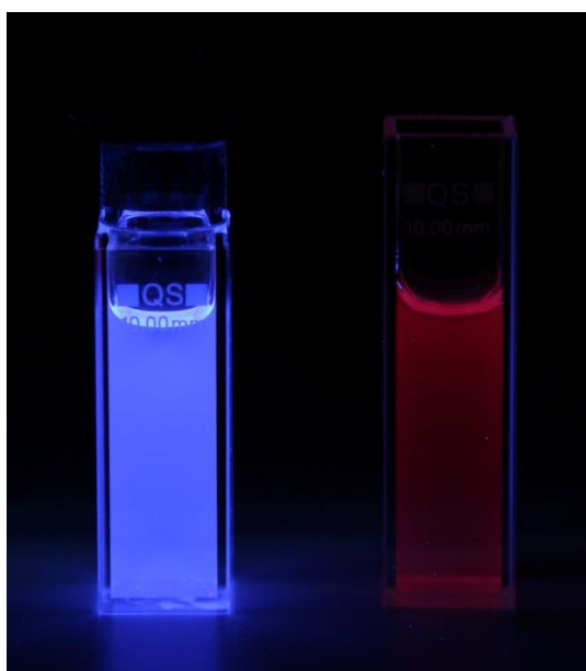
Figure 3-11 Dissolved conjugated polymers (left) and conjugated polymer-based nanoparticles (right) under UV light.
