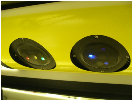
Figure 7.19: BB2FLSV4 and BB2FLSV5 sensors installed in a Slocum Glider.
