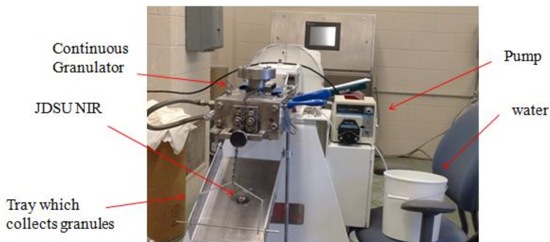
Figure 5.1 Inline monitoring set-up with tray
