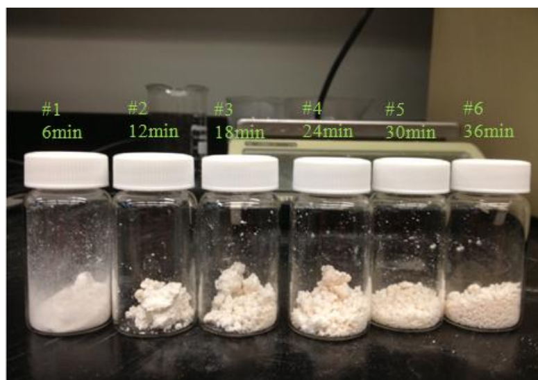
Figure 4.3. Samples shows the granulation process
