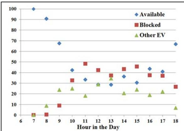
Figure 9: Probability of occupancy as a function of time of day for the CAIT locations. The groupings are rounded down: thus, the 9 O’Clock entry includes all data points through 9:59.
