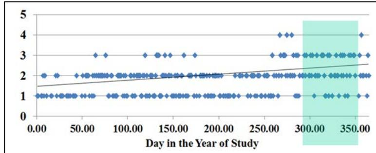
Figure 12: Peak simultaneous usage of the four available plug-in spots. The shaded region covers a time when one of the Level-2 chargers was broken, so the maximum possible during that period was three.
