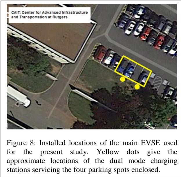
Figure 8: Installed locations of the main EVSE used for the present study. Yellow dots give the approximate locations of the dual mode charging stations servicing the four parking spots enclosed.
