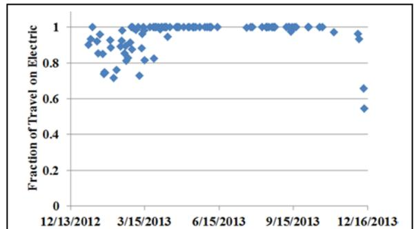
Figure 6: Fraction of simple round-trip commute cycles powered completely on electricity.
