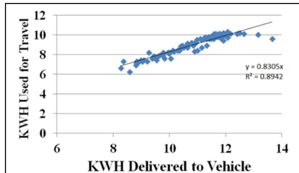
Figure 3: Round-trip electric energy recovery after storage in the vehicle battery.
