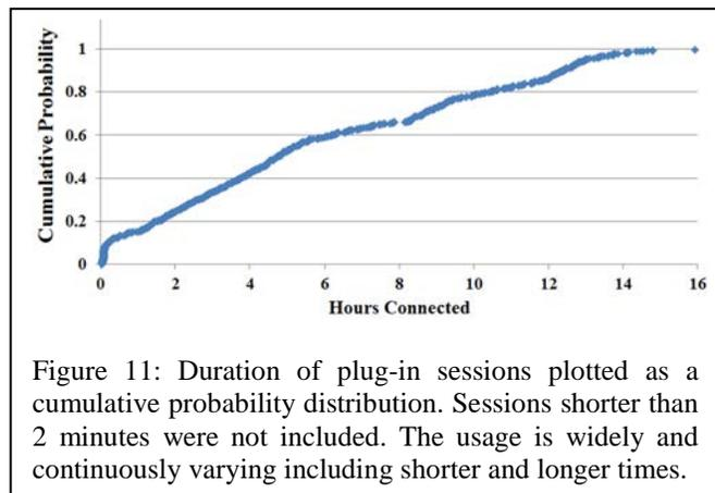
Figure 11: Duration of plug-in sessions plotted as a cumulative probability distribution. Sessions shorter than 2 minutes were not included. The usage is widely and continuously varying including shorter and longer times.
