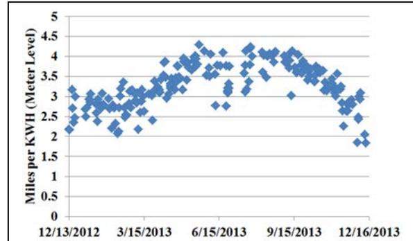
Figure 1: Miles traveled per KWH of energy metered at grid source level, through the year 1 testing period.
