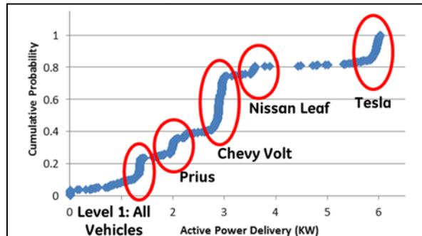
Figure 13: Cumulative probability distribution of the active power provided for each charging session. The specific humps represent vehicle types as marked.
