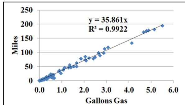
Figure 2: Miles traveled as a function of the quantity of gasoline used. The least-squares slope gives the miles-per-gallon rating for this vehicle.
