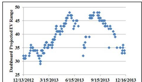
Figure 5: Vehicle’s projected range logged at each battery refill event during test period.
