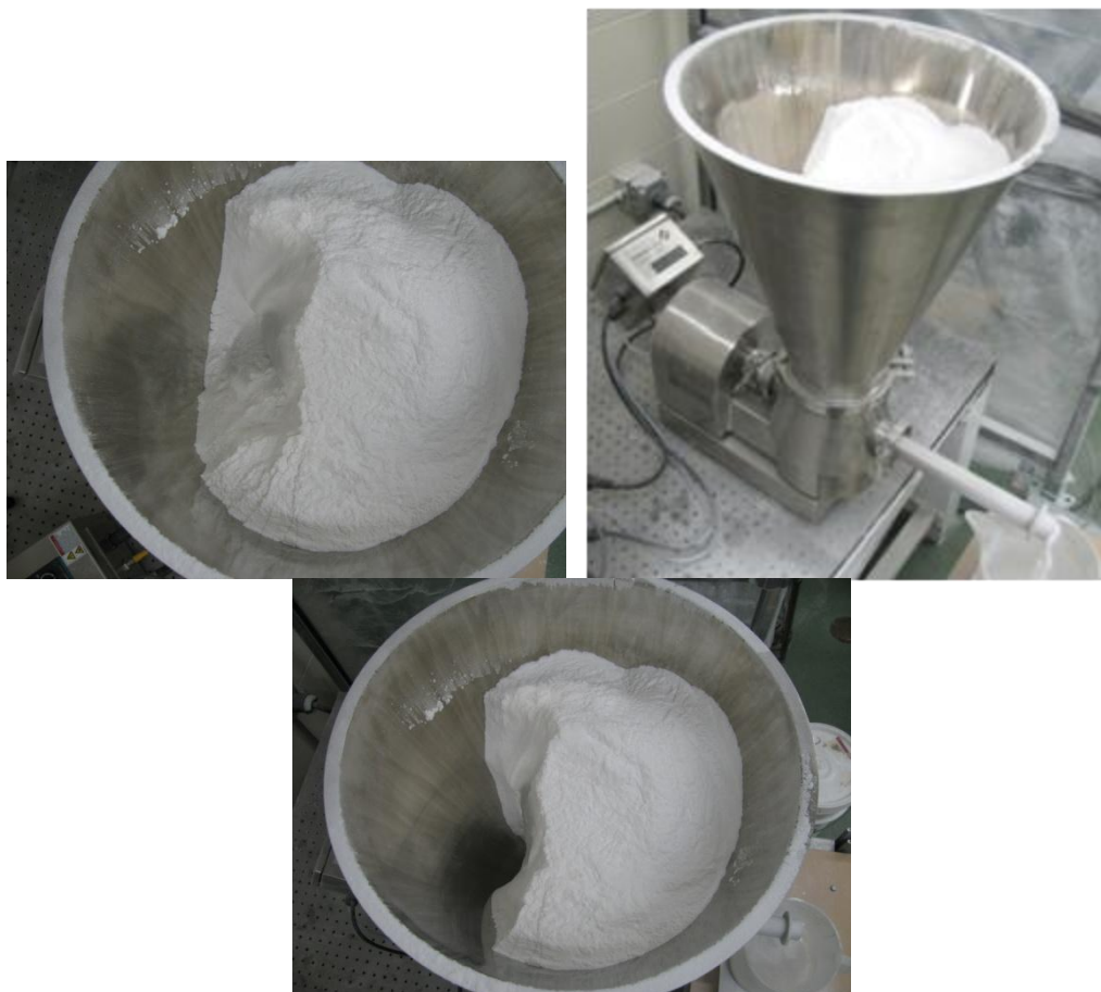
Figure 2.12: “Rat holing” and bridging shown in the hopper of a Schenck Accurate Purefeed feeder feeding a very cohesive powder.
