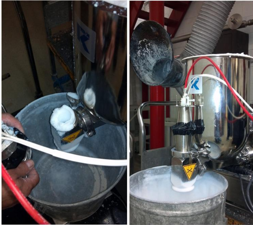
Figure 3.12: Picture of feeder (a) without static eliminator and (b) with static eliminator
