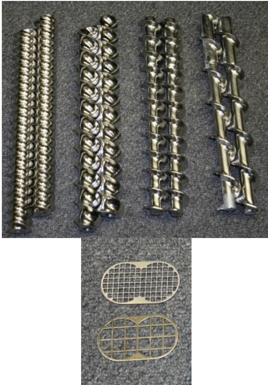
Figure 2.2: K-Tron KT35 feeder tooling. Consists of 4 sets of twin screws: fine concave screw (FCS), coarse concave screw (CCS), fine auger screw (FAS), and coarse auger screw (CAS). There are two screen: fine square screen (FSqS) and coarse square screen (CSqS). The feeder can also be run without a screen (NoS).
