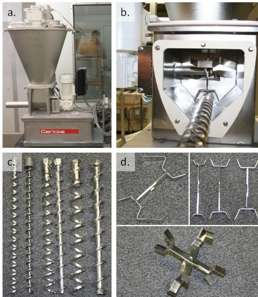
Figure 4.4: a.) Side-view of the Gericke GLD87 feeder; b.) Front view of the GLD87 with the faceplate and nozzle removed for a visual of the screw and agitator internal arrangement; c.) Various screws for the GLD87: Size 2 (Helix & Auger), Size 3 (Helix & Auger), and Size 4 (Helix & Auger); d.) Common agitator blade (top left), screw specific agitator blades (top right) and the combined agitator assembly (bottom)
