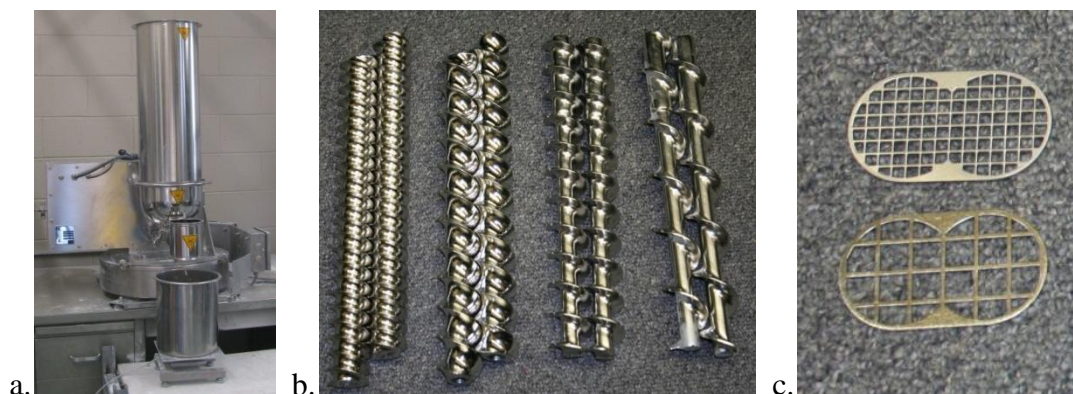
Figure 4.3: a.) KTron KT35 feeder with Schenck Accurate AccPro II catch scale. KTron KT35 feeder tooling consists of b.) 4 sets of twin screws: fine concave screw (FCS), coarse concave screw (CCS), fine auger screw (FAS), and coarse auger screw (CAS). c.) There are two screens: fine square screen (FSqS) and coarse square screen (CSqS). The feeder can also be run without a screen (NoS).
