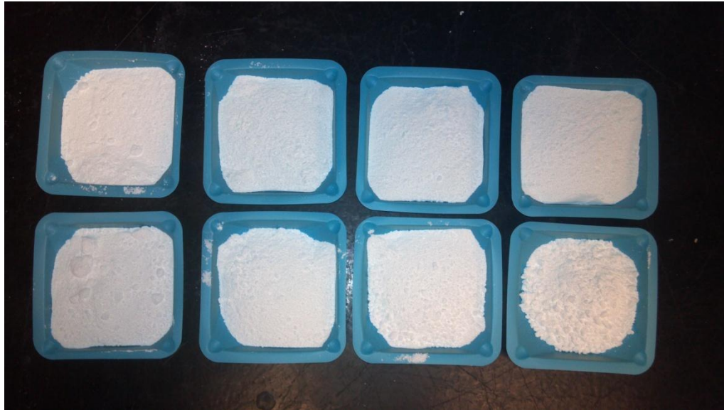
Figure 4.19: Samples showing the visual effects of feeding caused by various discharge screen conditions on zinc oxide powders. The top row is the Grillo material and the bottom row is the Norzinco material. From left to right (lowest shear to highest) is the bulk virgin powder, fed without a screen, fed with the coarse square screen, and fed with the fine square screen.
