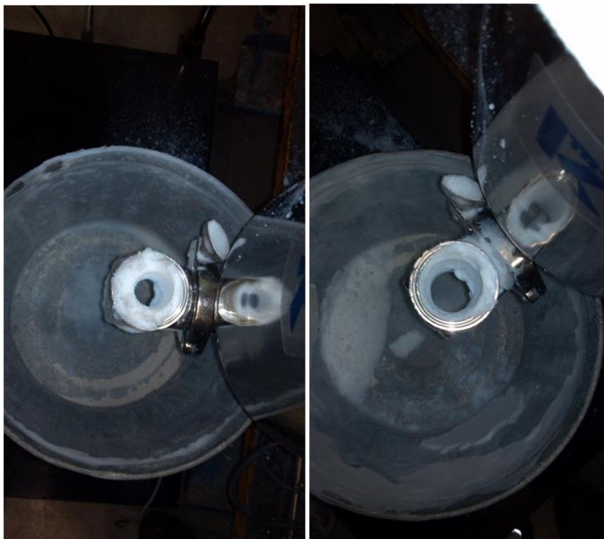
Figure 3.13: Picture of silicon dioxide buildup for (a) without static eliminator and (b) with static eliminator
