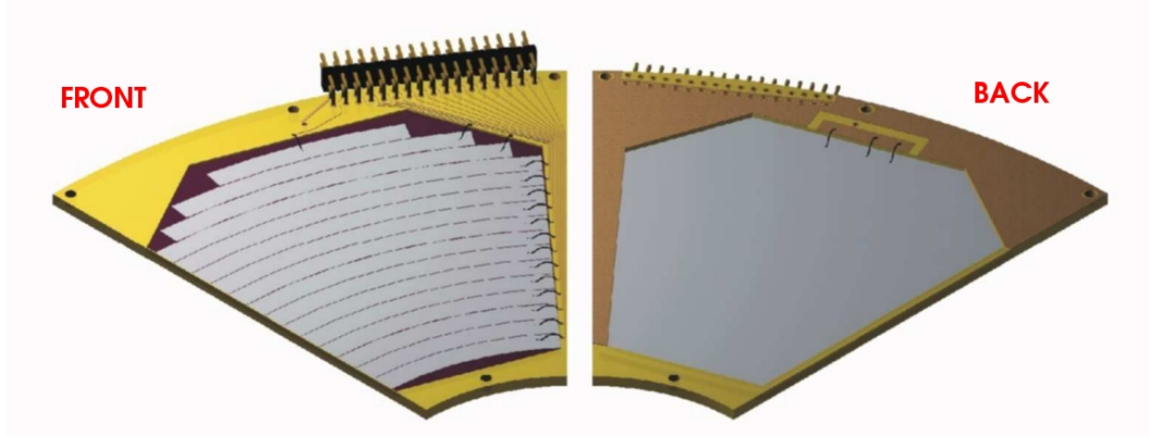
Figure 3.5: MSL-YY1 style detector used in the SIDAR array. Each detector has 16 annular non-resistive silicon strips on the front side and the back side is a single silicon pad.
