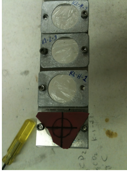
Figure 3.2: Deuterated polyethylene targets mounted on target drive for ^{124,126,128}\text{Sn}(d, p) reaction measurements at the HRIBF. Below the targets a phosphor is mounted for tuning the beam to the target chamber.
