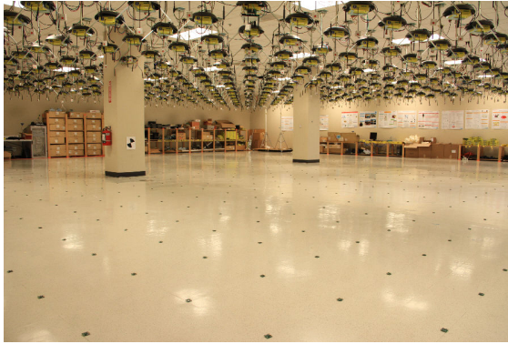
(a) Sensors at the ORBIT testbed facility arranged in a 24x24 regular grid on the floor. The computers overhead are ORBIT nodes used for the experiments.
