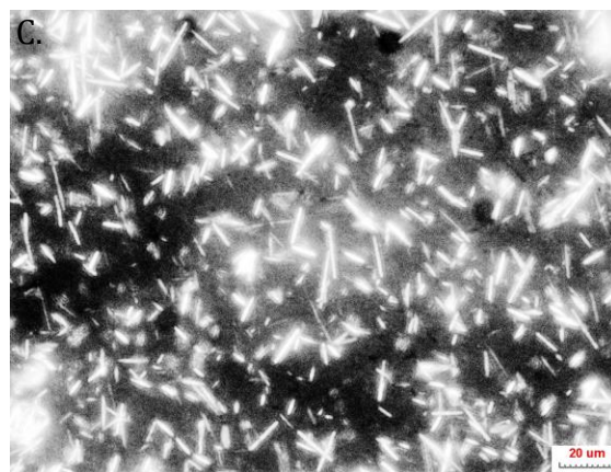
Figure 2.7 (A) Dynamic viscosities vs. angular frequency ( \omega ) for empty emulsion ( \times ), tangeretin emulsion ( \Delta ), and 5-demethyltangeretin emulsion (o). Microscopy images (40x) of 1:1 dilution of (B) 5-demethyltangeretin emulsion and (C) tangeretin emulsion, respectively. Emulsions were prepared with 52.5% MCT, 1.5% lecithin, 2.1% PMF compound, and 43.9% water.
