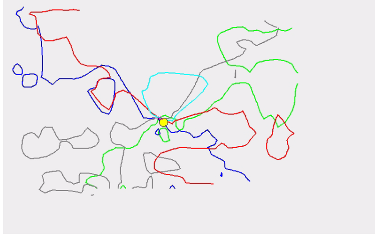
Figure 4.2: Example localization. Iso-RSS lines, 5-th and 4-th degree intersection areas for “best” localized points. Research lab data set. The minimum intersection area is basically a single point.
