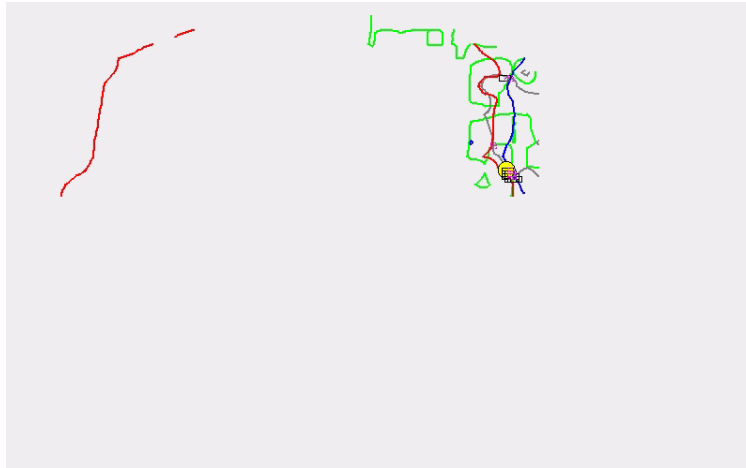
Figure 4.3: Example localization. Iso-RSS lines, 5-th and 4-th degree intersection areas for “best” localized points. CoRE3 data set. Although there are multiple minimum intersection areas, they are very small and close together.
