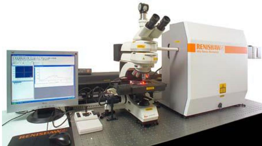
Figure 24. Renishaw InVia Confocal Micro-Raman Spectrometer (image courtesy Renishaw PLC).
