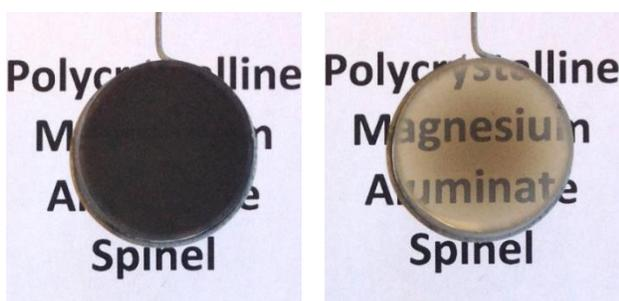
Figure 39. Photographs showing the appearance of samples heated at the rate of (a) 100°C/min, and (b) 10°C/min. The samples had a thickness of about 3 mm and were placed at 40 mm above the text.
