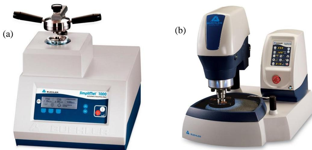
Figure 16. Buehler mounting press and polisher. (a) SimpliMet® 1000 Automatic Mounting Press; (b) EcoMet 250 Grinder-Polishers with AutoMet 250 Power Heads (picture courtesy Buehler, An ITW Company)
