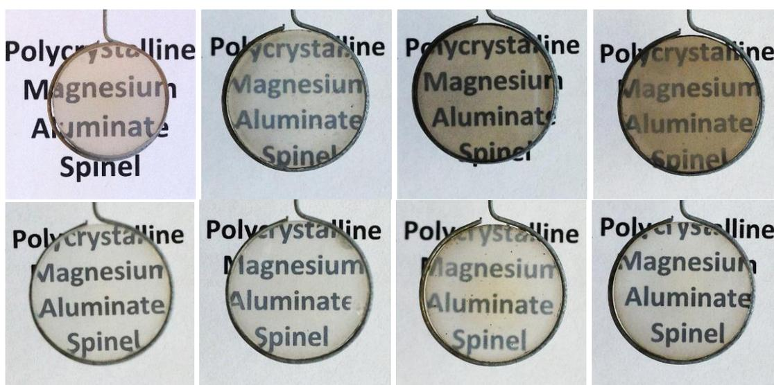
Figure 59. Illustration of the transparency of alumina doped samples. From the left: S0A, S1A, S3A, and S5A. The samples on the first row were SPS without the alumina protective layer. The samples on the second row were SPS with the alumina protective layer.
