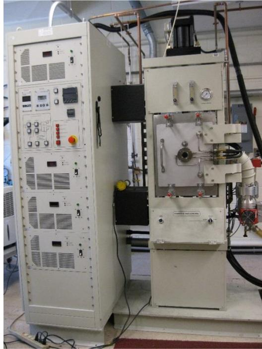
Figure 13. Thermal Technology's spark plasma sintering system.
