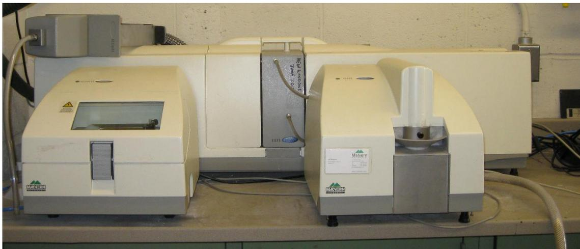
Figure 18. Malvern Mastersizer 2000 Light Scattering Particle Sizer with Scirocco Dry Powder Feeder (front left) and Hydro S Small Volume Wet Dispersion Cell (front right) accessories.
