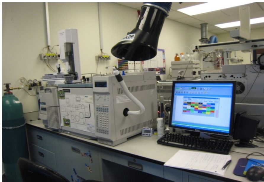
Figure 11. Gas Chromatograph-Mass Spectrometer equipped with sniff port for GC-O analysis.
