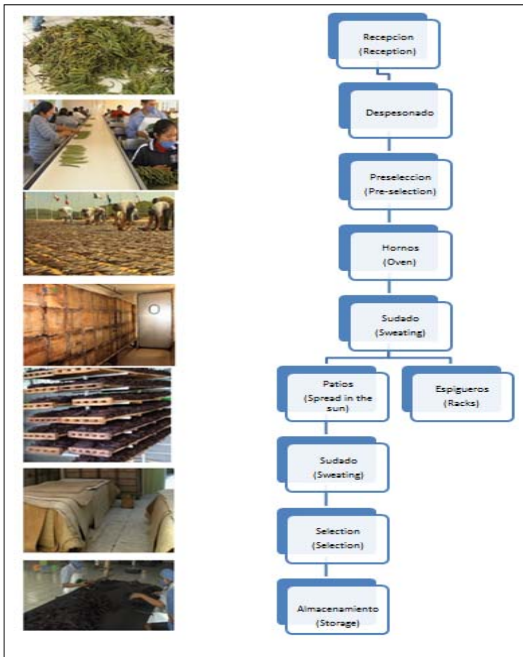
Figure 43. Mexican Curing Process (Beneficiado) workflow. Diagram and pictures courtesy of Desarrollo Agroindustrial Gaya, S.A. de C.V ( www.vanillamexico.com ).
