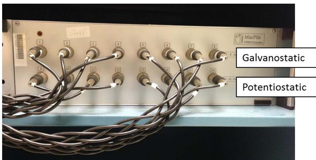
Figure 2.4. Macpile unit contain 16 channels used for testing cells. Ch. 1-8 is for galvanostatic tests and Ch. 9-16 is for potentiostatic tests.
