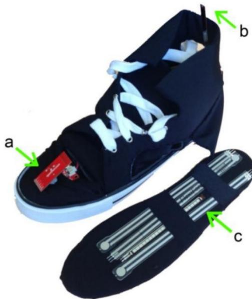
**Figure 2.9:** Instrumented shoe from Smartxa Project: (a) inertial measurement unit; (b) flexible goniometer; and (c) pressure sensors which are situated inside the insole.
