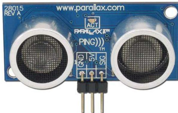
**Figure 2.13:** Active Ultrasonic sensor.
