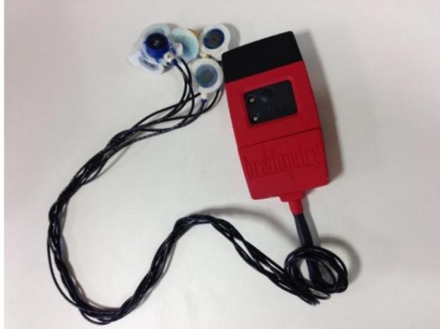
**Figure 2.14:** Brain query Wireless EMG/EEG/ECG system.
