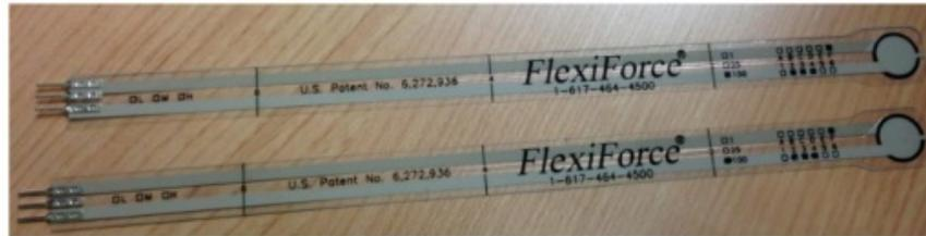
**Figure 2.8:** FlexiForce piezoresistive pressure sensor.
