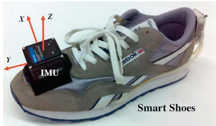
**Figure 2.10:** A tele-monitoring system for gait rehabilitation with Smart Shoes and an IMU (Borrowed from Bae et al. [36]).
