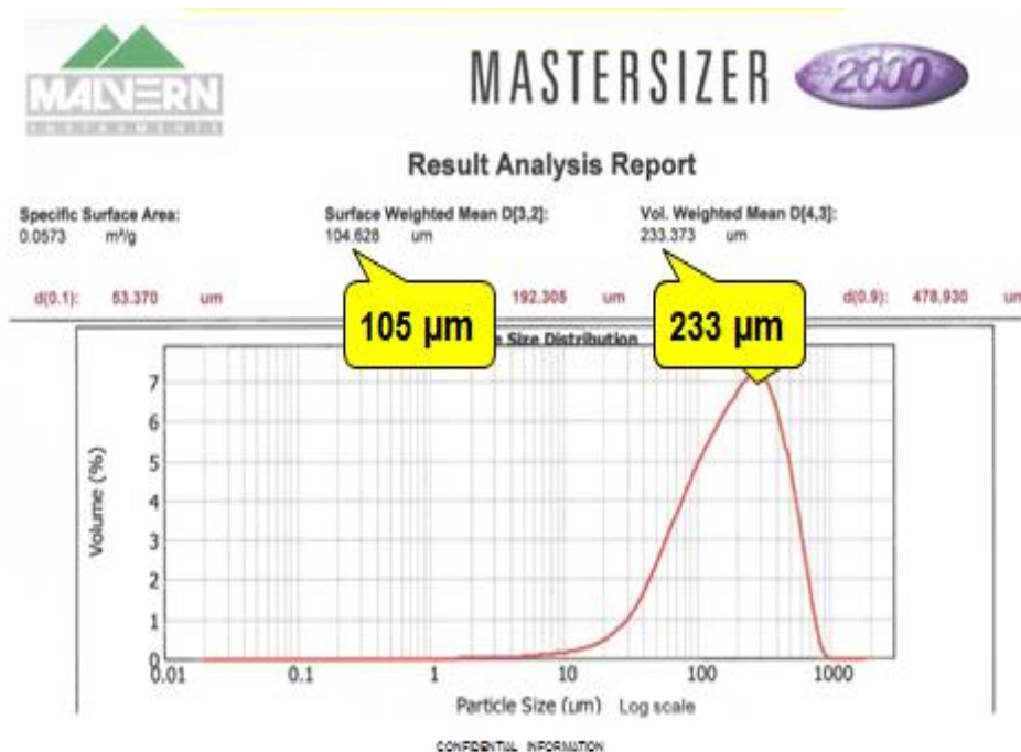
Figure 8. Particle Size Distribution via Malvern Analyzer
