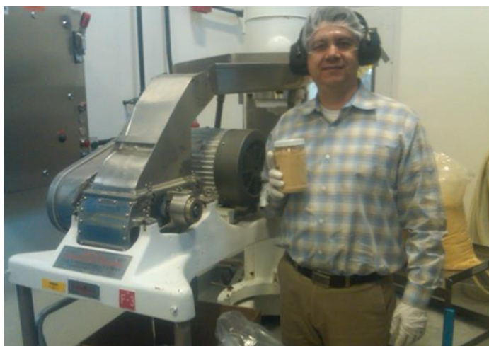
Figure 6. Micronization via FitsMill
