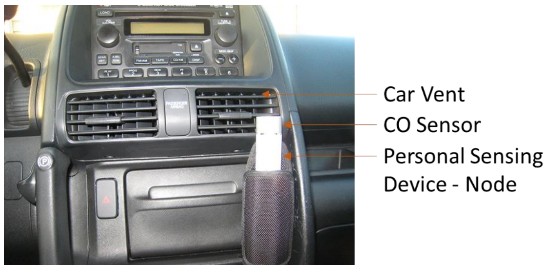
Figure 2-0-7 Node Sensor Setup Inside Car
