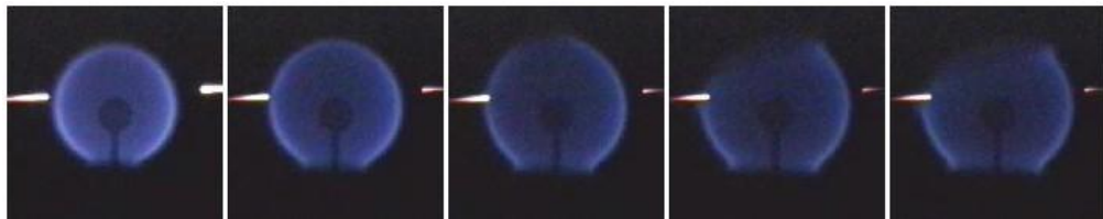
Figure 1.1: Spherical diffusion flame images from 5.0-s drop tower, showing the onset of radiative extinction. 2
