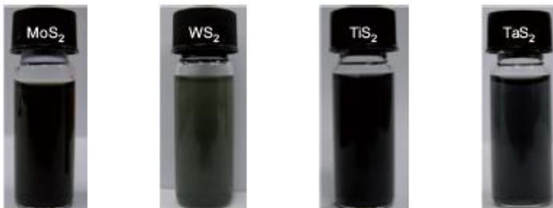
**Fig 3.6: TMDs prepared by lithium intercalation based exfoliation. Reproduced from Ref. 14.**
