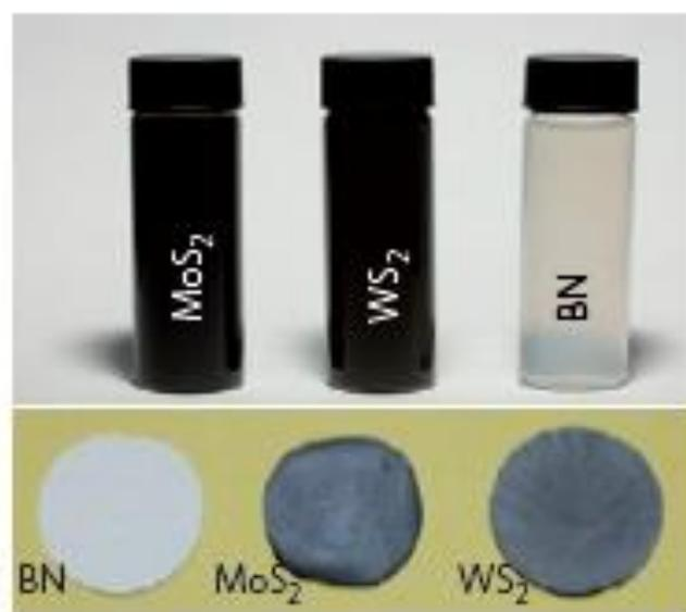
**Fig 3.5: TMD Solutions prepared by ultra-sonication with organic solvents and corresponding films. Reproduced from Ref. 118**
