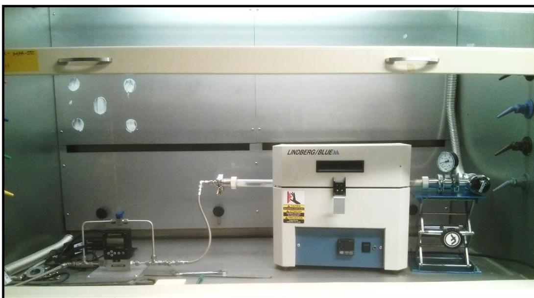
**Fig 8.1. Photograph of the furnace used for the growth of chemical vapor deposition of MoS<sub>2</sub>**
