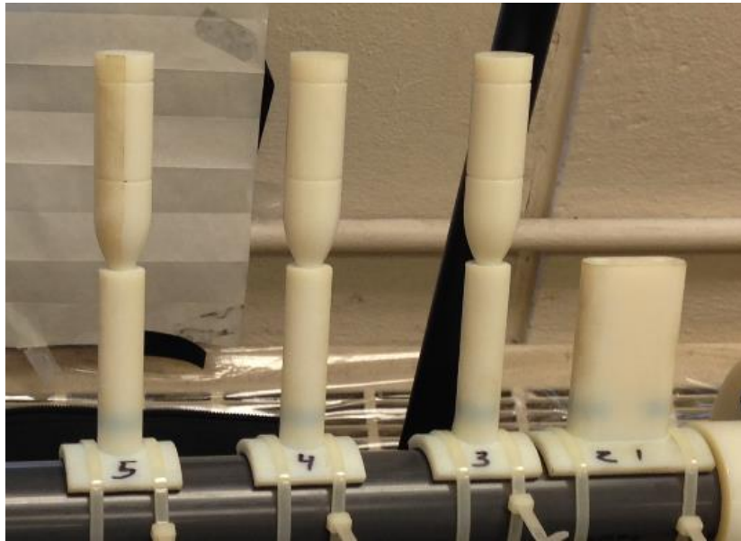
Figure 3.2 3D Printed Microphone Holders Attached to Multiple Microphone Positions
