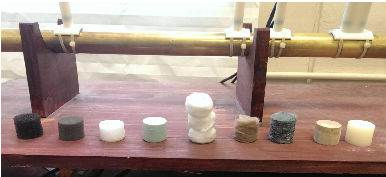
Figure 5.1 Samples Tested ( from left to right, Foam Matrix, Polyurethane, Melamine, Green Foam, Cotton, Fiberglass, Denim, Pine, Acrylic)
