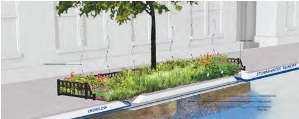
**Figure 1-2:** NYC Bioswale Example. (NYC DEP. Types of Green Infrastructure. 2014. [www.nyc.gov/html/dep/html/stormwater/combined\\_sewer\\_overflow\\_bmps.shtml](http://www.nyc.gov/html/dep/html/stormwater/combined_sewer_overflow_bmps.shtml))
