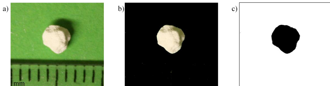
Figure 43. Image analysis process for granule sizing, showing (a) the optical image of the granule, (b) the background of the image removed, and (c) the granule pixilated for measurement of pixel area.
