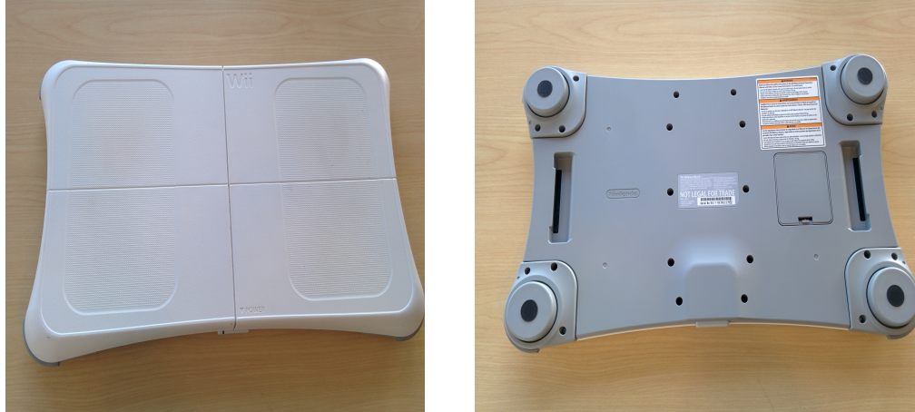
(a) Wii Balance Board front side. The design is similar to bathroom scales. (b) Wii Balance Board back side. Four sensors are provided at four corners of the board.
