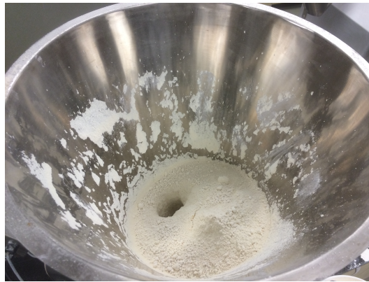
Figure 3-19 a hole create when feeding satintone
