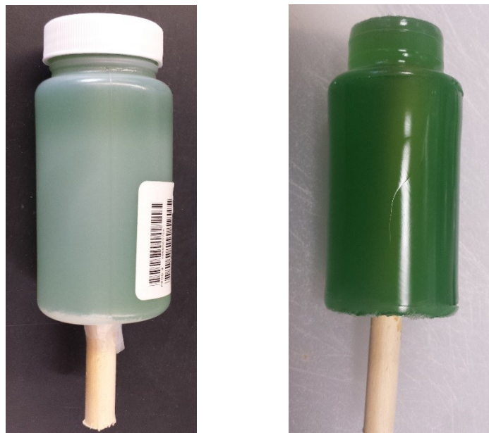
Figure 4.2: Gelatin-agar gel model system with a single inclusion, inside the plastic jar (left) and outside the jar (right).
