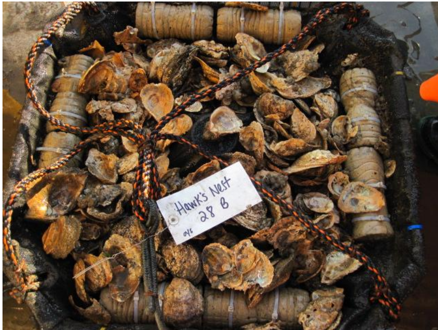
Fig. 3. A benthic habitat tray ( 0.36 \text{ m}^2 \times 9.5 \text{ cm} high) filled with substrate post-deployment. Weights are concrete cylinders zip-tied to the sides of the plastic, lined trays.
